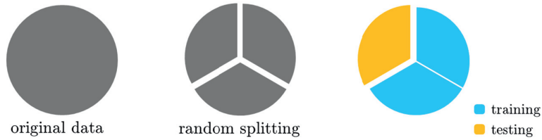
Fig. 5.15 Hold out cross-validation. The original data (left panel) shown here as the entire circular mass is split randomly (middle panel) into k non-overlapping sets (here k = 3 ). (right panel) One piece, or 1/k of the original dataset, is then taken randomly as the testing set with the remaining pieces, or k-1/k of the original data, taken as the training set.
